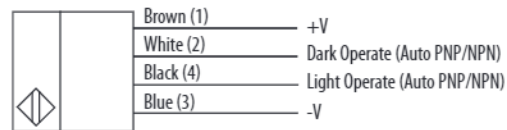
Figure 3 - Transmitted Beam Receiver (42AF-R1MAB1-F4 and 42AF-R1MAB1-D4) Light Operate and Dark Operate (Auto PNP or NPN)
